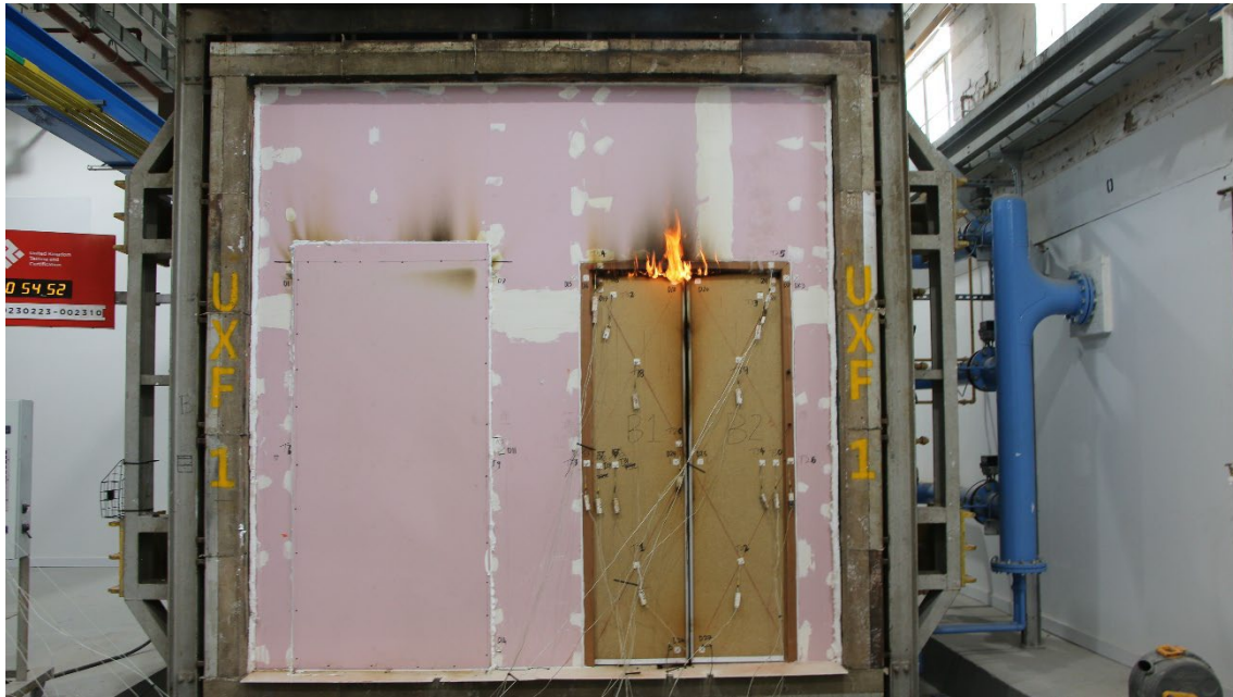
Figure 24 - The unexposed surface of the test construction after a test duration of 54 minutes
