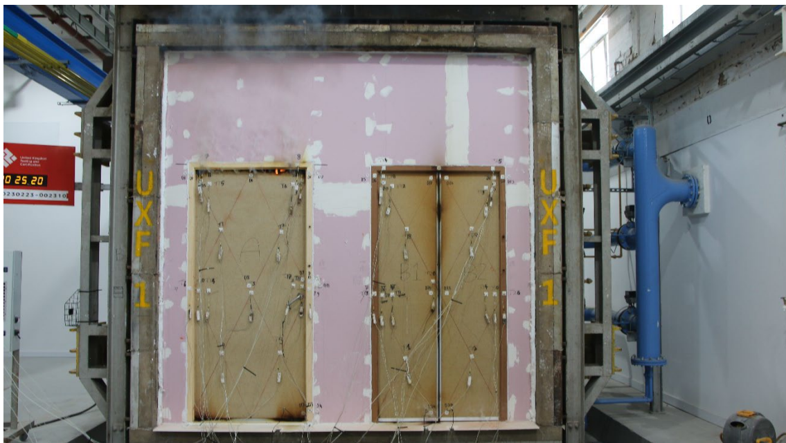
Figure 21 - The unexposed surface of the test construction after a test duration of 25 minutes
