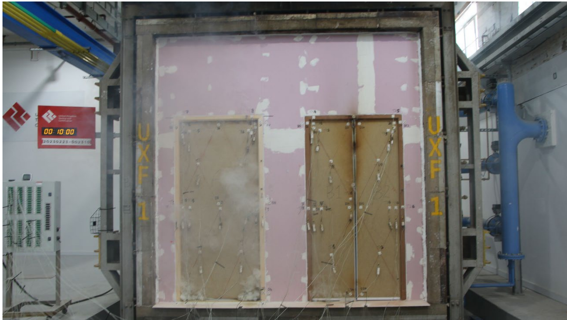
Figure 20 - The unexposed surface of the test construction after a test duration of 10 minutes
