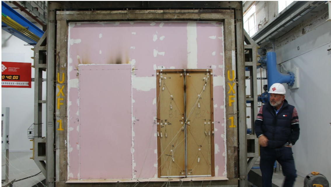
Figure 22 - The unexposed surface of the test construction after a test duration of 40 minutes
