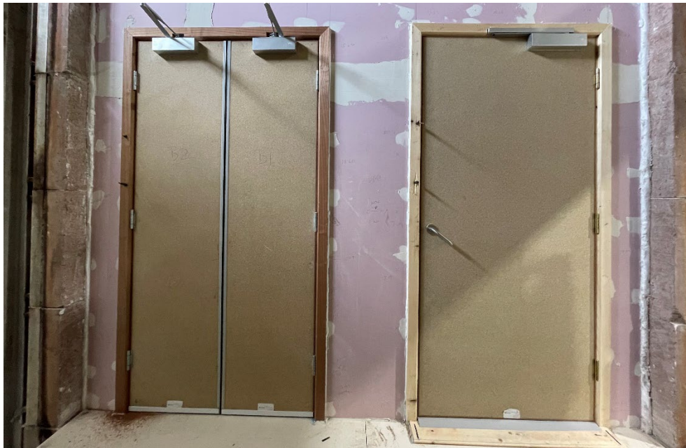
Figure 18 – The exposed surface of the test construction prior to commencement of the test
