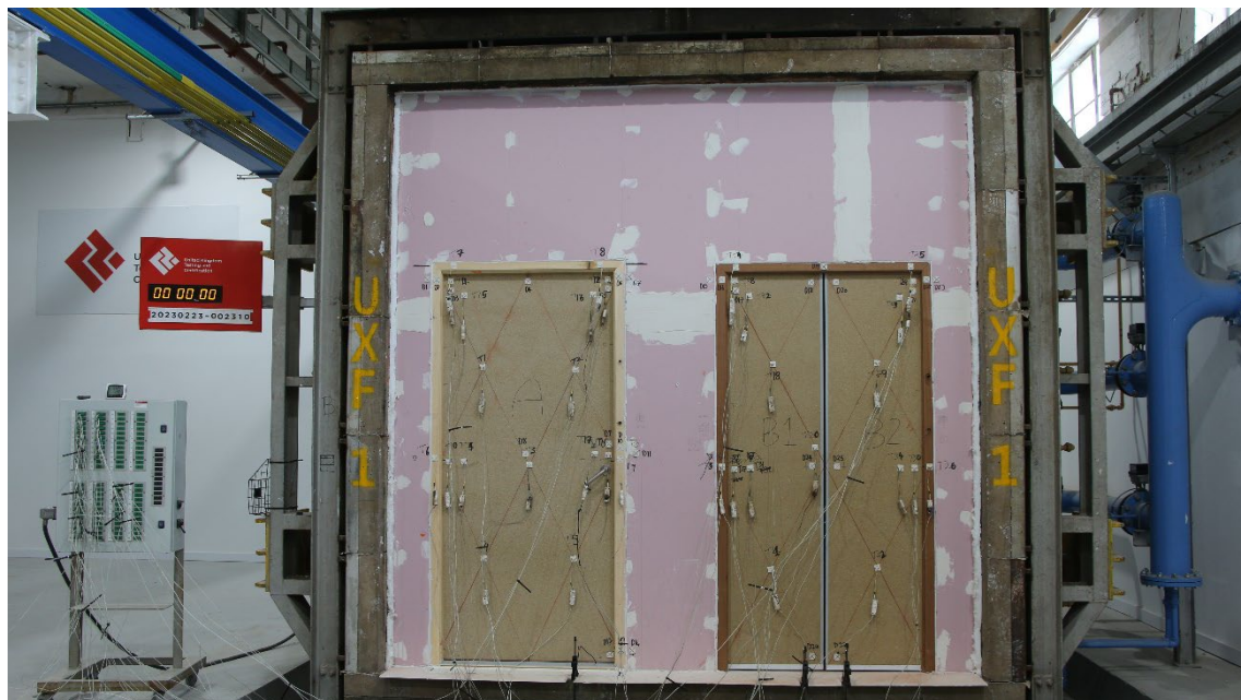
Figure 19 - The unexposed surface of the test construction prior to the commencement of the test
